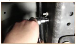
6. Remove the two 13mm bolts that connect the shield on the bottom of the frame rail.
