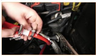
21. Install the tee fitting onto the factory lower heater hose you previously cut (step 19). Make sure the worm-gear clamps are already on the hose before installing the tee fitting. Tighten the worm-gear clamps. (flathead screwdriver)
