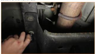
7. Slide the mounting bracket between the frame rail and the shield.
