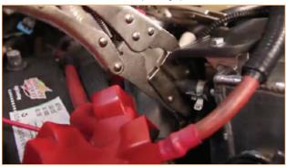
24. Cut the factory small coolant overflow line (hose cutters)
