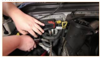
20. Attach a worm-gear clamp onto the shorter Mishimoto hose, connect the tee fitting, and tighten the worm-gear clamp. (flathead screwdriver)
