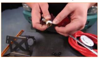
2. Thread the ball valves into the housing and tighten until they are seated properly. Do not overtorque the valves. (2x ball valves, 20mm wrench)
