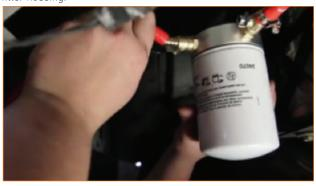
12. Route the Mishimoto hoses toward the front of your truck and up through the inner wheel well on the passenger side.
